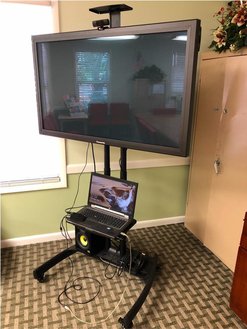
This station consists of a Flat Screen Monitor, a portable workstation, a wide angle webcam, and a powered speaker.
