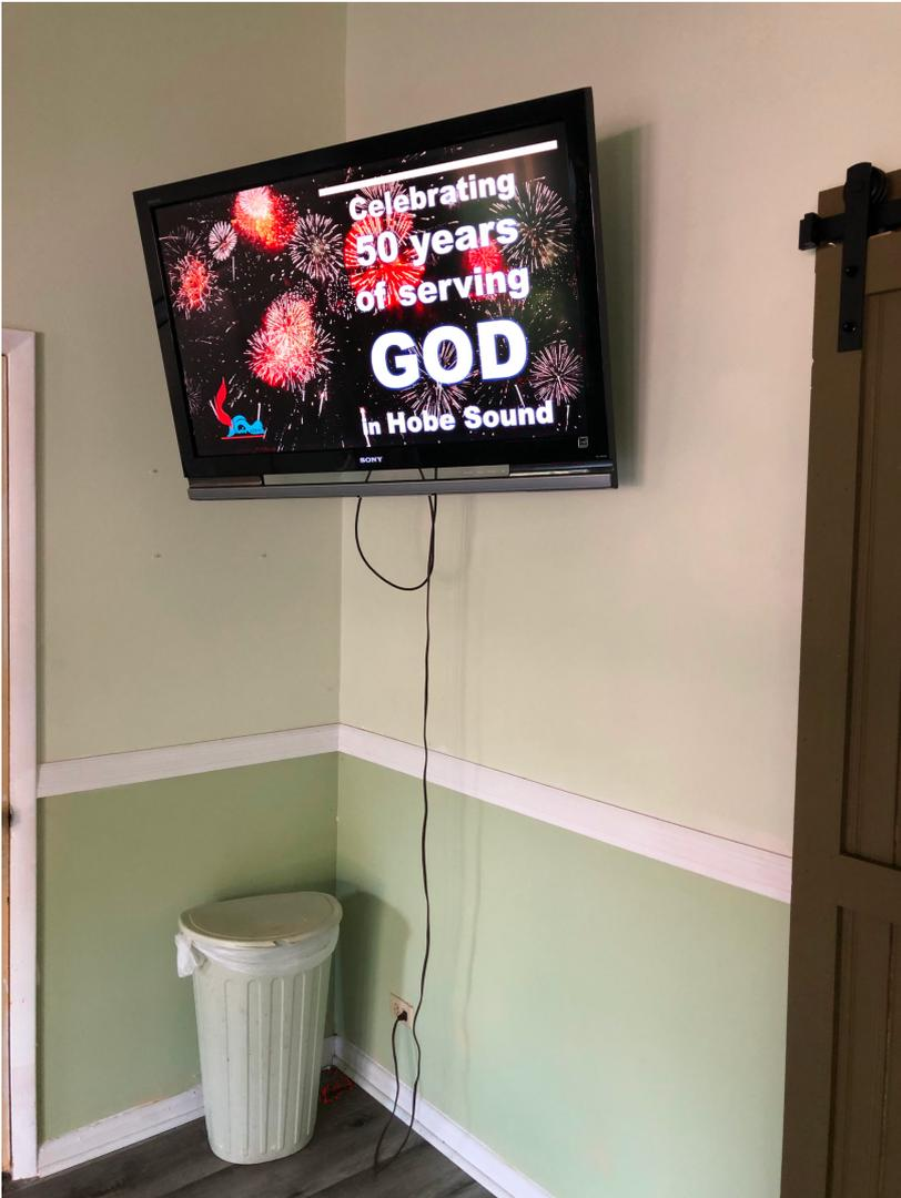
The station consists of a flat screen monitor and a connected Amazon Fire Stick. The Fire Stick is an adapter which permits the flat screen TV to perform as a "Smart" unit, with applications available. For this application we use the DS-Video application which connects to our file server to access video files.
